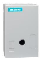
Non-reversing NEMA contactor, Size 0, Single phase full voltage, Contactor amp rating 18A, 3 wire (NO aux included), 24VAC 50-60Hz coil, Non-combination type, Enclosure NEMA type 1, Indoor general purpose use, Standard width enclosure
