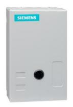
Non-reversing NEMA contactor, Size 0, Single phase full voltage, Contactor amp rating 18A, 3 wire (NO aux included), 220-240/440-480VAC 60Hz coil, Non-combination type, Enclosure NEMA type 1, Indoor general purpose use, Standard width enclosure
