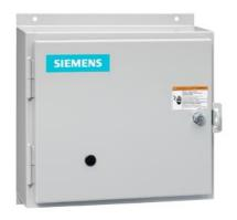
Non-reversing NEMA contactor, Size 0, Single phase full voltage, Contactor amprating 18A, 3 wire (NO aux included), 110V 50Hz / 120V 60Hz coil, Non-combination type, Enclosure NEMA type 12, Dust/drip proof for indoors, Standard width enclosure
