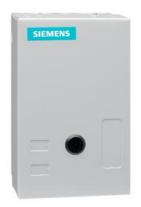
Non-reversing NEMA contactor, Size 00, Three phase full voltage, Contactor amprating 9A, 3 wire (NO aux included), 24VAC 50-60Hz coil, Non-combination type, Enclosure NEMA type 1, Indoor general purpose use, Standard width enclosure
