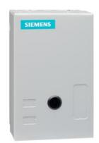
Non-reversing NEMA contactor, Size 00, Three phase full voltage, Contactor amp rating 9A, 3 wire (NO aux included), 380-440/440-480V 50/60Hz coil, Non-combination type, Enclosure NEMA type 1, Indoor general purpose use, Standard width enclosure
