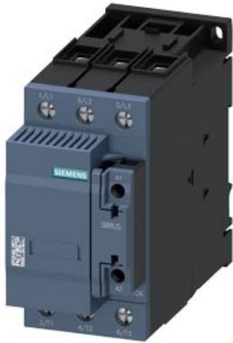
capacitor contactor, AC-6b 75 kVAr, / 400 V, 3-pole, 230 V AC, 50 Hz, auxiliary contacts: 1 NO + 1 NC, screw terminal, size: S2
