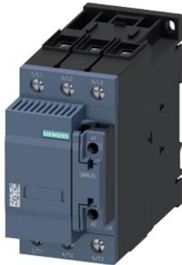
capacitor contactor, AC-6b 50 kVA<sub>r</sub>, / 400 V, 3-pole, 110 V AC, 50 Hz, auxiliary contacts: 2 NC, screw terminal, size: S2
