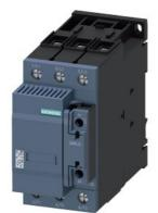
capacitor contactor, AC-6b 50 kVAr, / 400 V, 3-pole, 110 V AC, 50 Hz, auxiliary contacts: 1 NO + 1 NC, screw terminal, size: S2  $\,$
