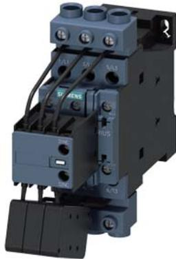
capacitor contactor, AC-6b 33 kVA<sub>r</sub>, / 400 V, 3-pole, 200-280 V AC/DC, 50/60 Hz, with integrated varistor, auxiliary contacts: 1 NO + 2 NC, screw terminal, size: S0
