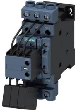
capacitor contactor, AC-6b 33 kVA<sub>r</sub>, / 400 V, 3-pole, 110 V DC, auxiliary contacts: 1 NO + 2 NC, screw terminal, size: S0
