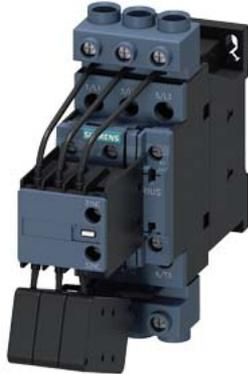
capacitor contactor, AC-6b 33 kVA<sub>r</sub>, / 400 V, 3-pole, 24 V AC, 50 Hz, auxiliary contacts: 1 NO + 2 NC, screw terminal, size: S0
