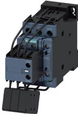
capacitor contactor, AC-6b 20 kVA<sub>r</sub>, / 400 V, 3-pole, 21-28 V AC/DC, 50/60 Hz, with integrated varistor, auxiliary contacts: 1 NO + 2 NC, screw terminal, size: S0
