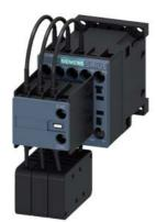
capacitor contactor, AC-6b 12.5 kVAr, / 400 V, 3-pole, 24 V DC, auxiliary contacts: 2 NC, screw terminal, size: S00
