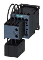
capacitor contactor, AC-6b 12.5 kVAr, / 400 V, 3-pole, 24 V AC, 50/60 Hz, auxiliary contacts: 1 NO + 1 NC, screw terminal, size: S00
