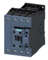
power contactor, AC-3, 51 A, 22 kW / 400 V, 4-pole, 20-33 V AC/DC, 50/60 Hz, with integrated varistor, main contacts: 2 NO + 2 NC, auxiliary contacts: 1 NO + 1 NC, screw terminal, size: S2
