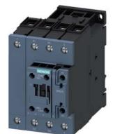
power contactor, AC-3, 51 A, 22 kW / 400 V, 4-pole, 230 V AC, 50 Hz, main contacts: 2 NO + 2 NC, auxiliary contacts: 1 NO + 1 NC, screw terminal, size: S2
