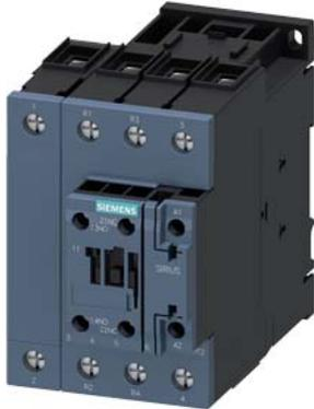
power contactor, AC-3, 51 A, 22 kW / 400 V, 4-pole, 24 V AC, 50/60 Hz, main contacts: 2 NO + 2 NC, auxiliary contacts: 1 NO + 1 NC, screw terminal, size: S2
