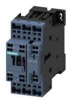
traction contactor, AC-3, 25 A, 11 kW / 400 V, 4-pole, 72 V DC, 0.7-1.25\* Us, electronic drive, with integrated varistor, main contacts: 2 NO + 2 NC, auxiliary contacts: 1 NO + 1 NC, spring-loaded terminal, size: S0
