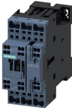
power contactor, AC-3, 25 A, 11 kW / 400 V, 4-pole, 220 V DC, main contacts: 2 NO + 2 NC, auxiliary contacts: 1 NO + 1 NC, spring-loaded terminal, size: S0
