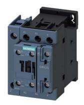
power contactor, AC-3, 25 A, 11 kW / 400 V, 4-pole, 110 V AC, 50/60 Hz, main contacts: 2 NO + 2 NC, auxiliary contacts: 1 NO + 1 NC, screw terminal, size: S0
