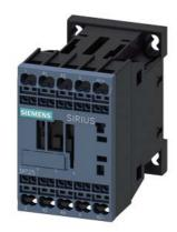
power contactor, AC-3, 16 A, 7.5 kW / 400 V, 4-pole, 220 V DC, main contacts: 2 NO + 2 NC, spring-loaded terminal, size: S00
