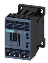
power contactor, AC-3, 16 A, 7.5 kW / 400 V, 4-pole, 110 V AC, 50 Hz / 120 V, 60 Hz, main contacts: 2 NO + 2 NC, spring-loaded terminal, size: S00
