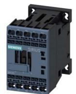
power contactor, AC-3, 12 A, 5.5 kW / 400 V, 4-pole, 48 V DC, main contacts: 2 NO + 2 NC, spring-loaded terminal, size: S00
