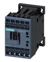
power contactor, AC-3, 12 A, 5.5 kW / 400 V, 4-pole, 110 V AC, 50 Hz / 120 V, 60 Hz, main contacts: 2 NO + 2 NC, spring-loaded terminal, size: S00
