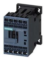
power contactor, AC-3, 12 A, 5.5 kW / 400 V, 4-pole, 24 V AC, 50/60 Hz, main contacts: 2 NO + 2 NC, spring-loaded terminal, size: S00
