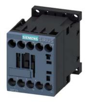
power contactor, AC-3, 12 A, 5.5 kW / 400 V, 4-pole, 220 V DC, main contacts: 2 NO + 2 NC, screw terminal, size: S00  $\,$
