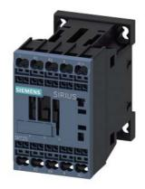
power contactor, AC-3, 9 A, 4 kW / 400 V, 4-pole, 220 V DC, main contacts: 2 NO + 2 NC, spring-loaded terminal, size: S00  $\,$
