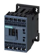
power contactor, AC-3, 9 A, 4 kW / 400 V, 4-pole, 110 V AC, 50 Hz / 120 V, 60 Hz, main contacts: 2 NO + 2 NC, spring-loaded terminal, size: S00
