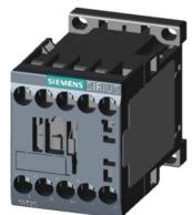
power contactor, AC-3, 9 A, 4 kW / 400 V, 4-pole, 48 V AC, 50/60 Hz, main contacts: 2 NO + 2 NC, screw terminal, size: S00
