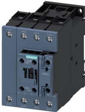
contactor AC-1, 110 A, 400 V / 40 °C, 4-pole, 230 V AC, 50 Hz, auxiliary contacts: 1 NO + 1 NC, screw terminal, size: S2
