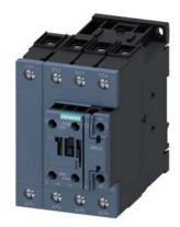
contactor AC-1, 60 A, 400 V / 40 °C, 4-pole, 83-155 V AC/DC, 50/60 Hz, with integrated varistor, auxiliary contacts: 1 NO + 1 NC, screw terminal, size: S2
