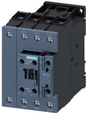
contactor AC-1, 60 A, 400 V / 40 °C, 4-pole, 110 V AC, 50 Hz / 120 V, 60 Hz, auxiliary contacts: 1 NO + 1 NC, screw terminal, size: S2
