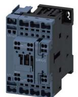
contactor AC-1, 40 A, 400 V / 40 °C, 4-pole, 220 V AC, 50 Hz / 240 V, 60 Hz, auxiliary contacts: 1 NO + 1 NC, spring-loaded terminal, size: S0
