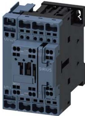
contactor AC-1, 40 A, 400 V / 40 °C, 4-pole, 24 V AC, 50 Hz, auxiliary contacts: 1 NO + 1 NC, spring-loaded terminal, size: S0
