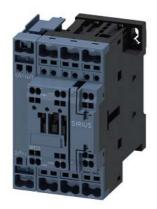
contactor AC-1, 35 A, 400 V / 40 °C, 4-pole, 230 V AC, 50 Hz, auxiliary contacts: 1 NO + 1 NC, spring-loaded terminal, size: S0
