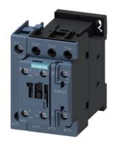
contactor AC-1, 35 A, 400 V / 40 °C, 4-pole, 230 V AC, 50/60 Hz, auxiliary contacts: 1 NO + 1 NC, screw terminal, size: S0
