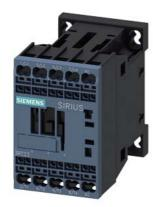
contactor AC-1, 22 A, 400 V / 40  $^{\circ}$ C, 4-pole, 220 V AC, 50 Hz / 240 V, 60 Hz, spring-loaded terminal, size: S00
