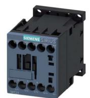
contactor AC-1, 22 A, 400 V / 40 °C, 4-pole, 12 V DC, screw terminal, size: S00
