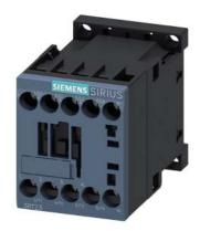
contactor AC-1, 22 A, 400 V / 40 °C, 4-pole, 110 V AC, 50/60 Hz, screw terminal, size: S00
