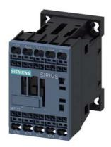
contactor AC-1, 18 A, 400 V / 40  $^{\circ}$ C, 4-pole, 110 V AC, 50 Hz / 120 V, 60 Hz, spring-loaded terminal, size: S00
