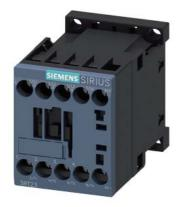
contactor AC-1, 18 A, 400 V / 40 °C, 4-pole, 12 V DC, screw terminal, size: S00  $\,$
