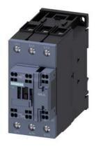
power contactor, AC-3e/AC-3, 80 A, 37 kW / 400 V, 3-pole, 230 V AC, 50/60 Hz, auxiliary contacts: 1 NO + 1 NC, main circuit: screw terminal, control and auxiliary circuit: spring-loaded terminal, size: S2, upright mounting position
