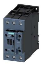
traction contactor, AC-3e/AC-3, 80 A, 37 kW / 400 V, 3-pole, 24 V DC, 0.7-1.25  $^{\star}$  Us, electronic drive, with integrated varistor, auxiliary contacts: 1 NO + 1 NC, screw terminal, size: S2
