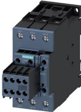
power contactor, AC-3e/AC-3, 80 A, 37 kW / 400 V, 3-pole, 20-33 V AC/DC, 50/60 Hz, with integrated varistor, auxiliary contacts: 2 NO + 2 NC, screw terminal, size: S2, removable auxiliary switch
