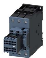
traction contactor, AC-3e/AC-3, 65 A, 30 kW / 400 V, 3-pole, 24 V DC, 0.7-1.25\* Us, electronic drive, with integrated varistor, auxiliary contacts: 2 NO + 2 NC, main circuit: screw terminal, control and auxiliary circuit: spring-loaded terminal, size: S2, removable auxiliary switch
