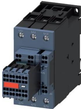
power contactor, AC-3e/AC-3, 65 A, 30 kW / 400 V, 3-pole, 20-33 V AC/DC, 50/60 Hz, with integrated varistor, auxiliary contacts: 2 NO + 2 NC, main circuit: screw terminal, control and auxiliary circuit: spring-loaded terminal, size: S2, captive auxiliary switch
