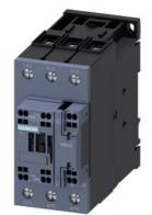
power contactor, AC-3e/AC-3, 65 A, 30 kW / 400 V, 3-pole, 24 V AC, 50/60 Hz, auxiliary contacts: 1 NO + 1 NC, main circuit: screw terminal, control and auxiliary circuit: spring-loaded terminal, size: S2
