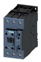
traction contactor, AC-3e/AC-3, 65 A, 30 kW / 400 V, 3-pole, 110 V DC, 0.7-1.25  $^{\star}$  Us, electronic drive, with integrated varistor, auxiliary contacts: 1 NO + 1 NC, screw terminal, size: S2
