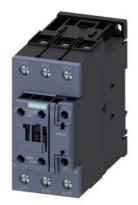
power contactor, AC-3e/AC-3, 65 A, 30 kW / 400 V, 3-pole, 220 V AC, 50 Hz / 240 V, 60 Hz, auxiliary contacts: 1 NO + 1 NC, screw terminal, size: S2
