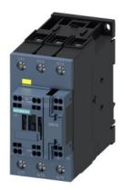
power contactor, AC-3e/AC-3, 51 A, 22 kW / 400 V, 3-pole, 83-150 V AC/DC, 50/60 Hz, with integrated varistor, auxiliary contacts: 1 NC, main circuit: screw terminal, control and auxiliary circuit: spring-loaded terminal, size: S2, F-PLC-IN
